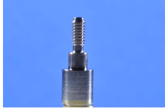
Figure 7 New healing abutment. Wiped, ultrasonic bath cleaned, sterilized, and stained with Phloxine B. No protein or peptide stained.
