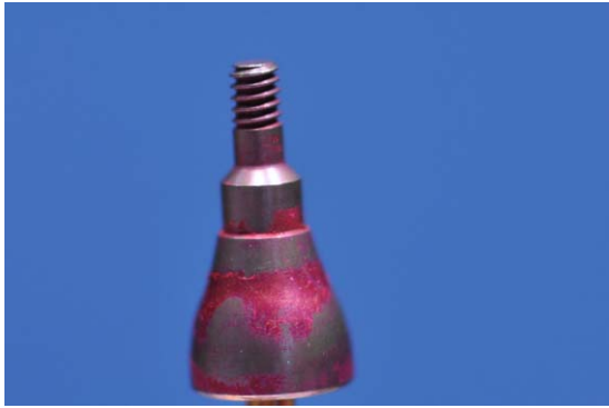
Figure 5 Anodized healing abutment, the phloxine B clearly highlights residual contamination site.
