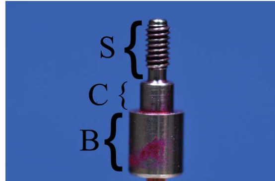
Figure 3 Site evaluation: B- Body of the abutment – represents three sections, (Implant, mid, occlusal) all show phloxine B staining and residual contamination. C- Connection to implant site. S- Screw thread shank and threads.
